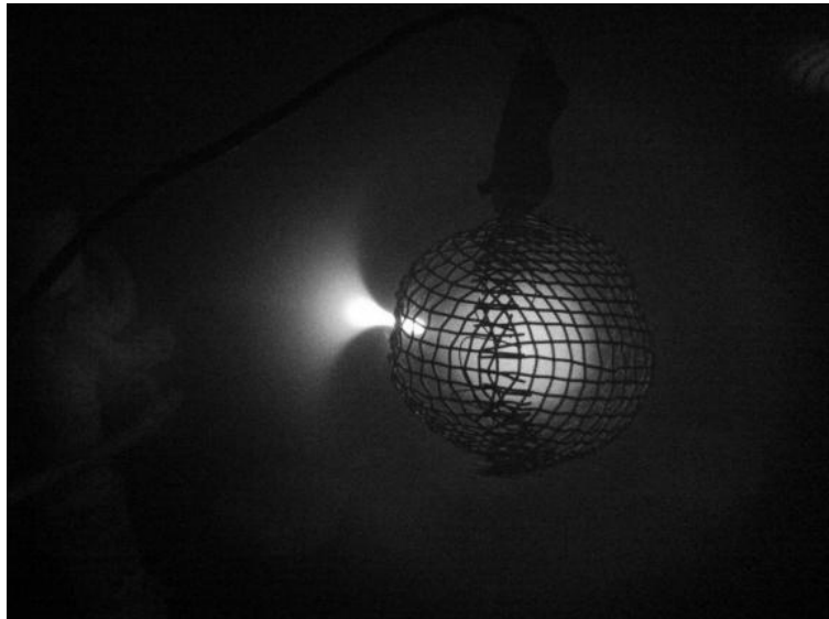
Fig. 4 – Photos of the complex space charge structures inside and around the cathode, in different stages of their development.
